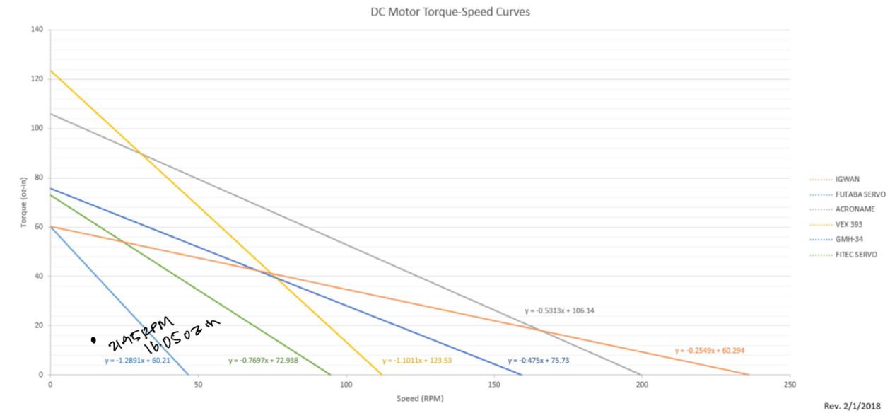
Figure 10: Speed/torque quantities for each motor
